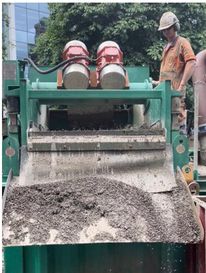
Figure 1 – A solids control unit
