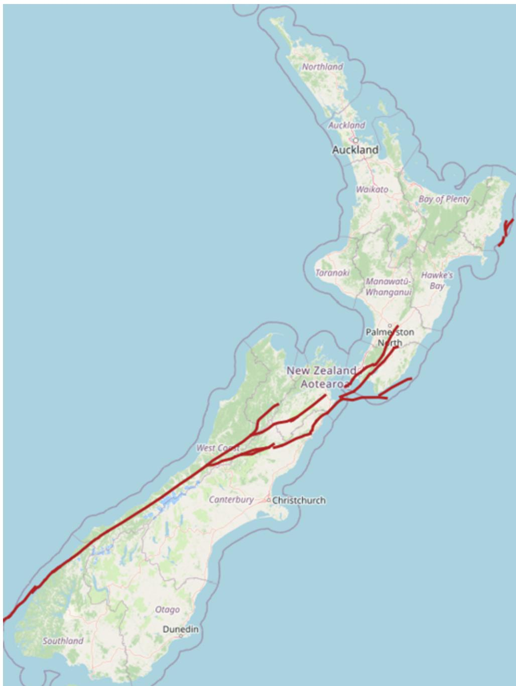
**Figure 3.2 – Major faults (faults listed in Table 3.2) requiring consideration of near-fault factors > 1.0**
